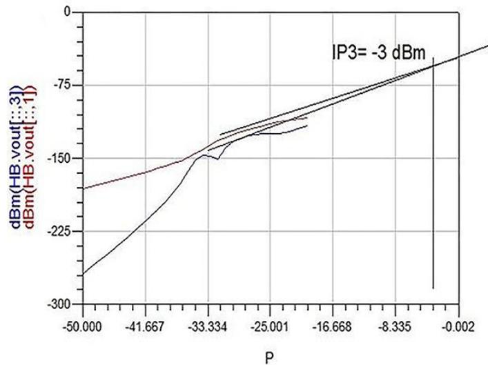
Fig. 11. IIP3 versus input power
