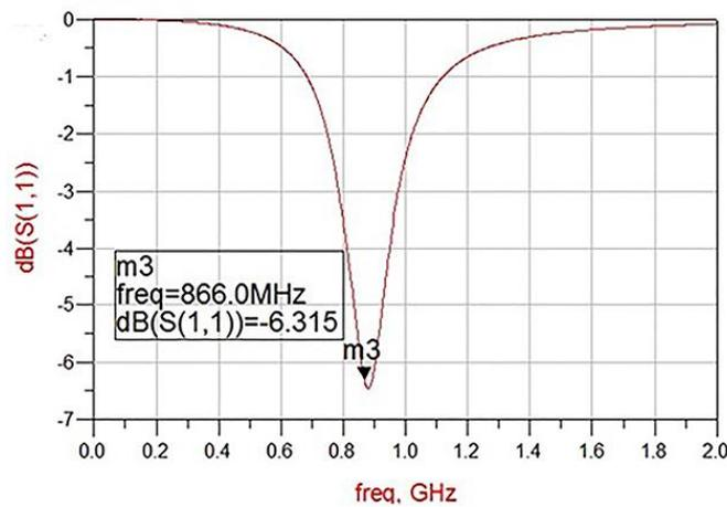
Fig. 8. Input return loss  $S_{11}$
