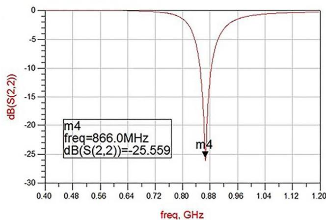
Fig. 9. Output return loss  $S_{22}$
