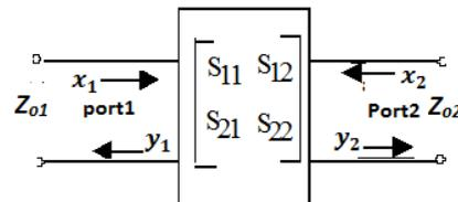
Fig. 2.  $S$  parameter of two-port network
