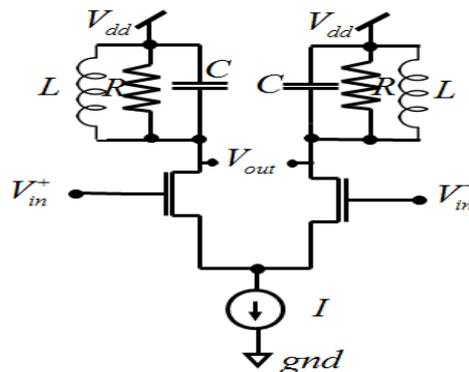
Fig. 4. Tuned LC amplifier circuit
