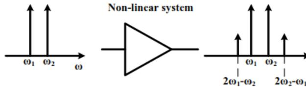
Fig. 3. Intermodulation in a nonlinear system
