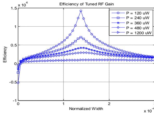
Fig. 5. Efficiency of tuned RF gain versus input transistor width
