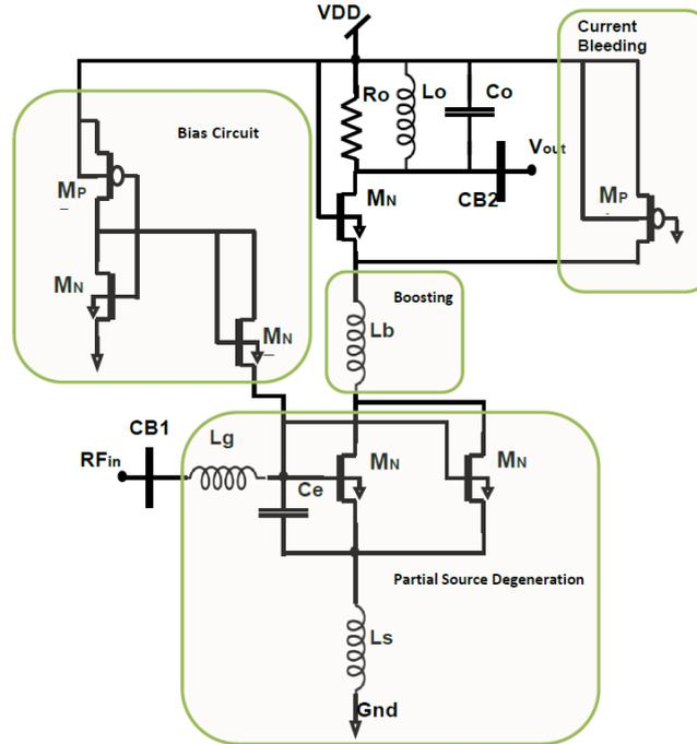
Fig. 6. The proposed 866MHz LNA schematic
