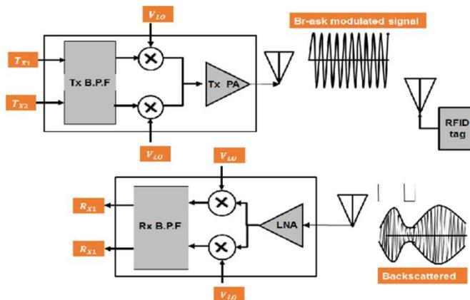
Fig. 1. The front-end block of a typical RFID reader
